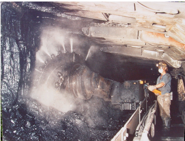
Figure 1 – A typical longwall shearer in operation underground.
